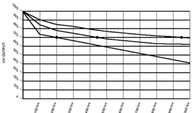
Lamp “A” loses 25% of its initial output in the first 100 hours and is down to 70% of initial output after only 200 hours of use. While this particular lamp may not have a place in a professional salon, it might be an acceptable lamp for use in a ‘home’ bed, particularly if it has a low cost.
