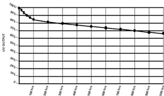
What is immediately apparent is the decline in output does not track in a straight linear path. The greatest decline takes place in about the first 100 hours. After the 100 hours, the rate of decline becomes less; there is a flattening out of the curve, but the decline in output still continues as the lamp burns. Although we call this a “maintenance curve” it is an imaginative stretch to call it a curve; the shape is more like a hockey stick.
