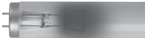
When all of the emissive coating is depleted, the cathodes (coils) are no longer capable of generating an electron flow, and the lamp is no longer able to start (it is “burned out”).
