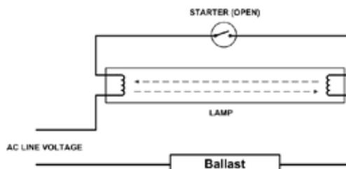
the heat causes the bi-metal contacts to bend and come together, closing the circuit.
