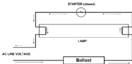
"Glo-bottle" starters (Cosmedico K11's and K12's or Philips S11's and S12's) are mechanical switches. They are constructed using bi-metal contacts housed within a neon filled glass bottle.
